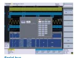
Search for portions of analysis results of the logic signal's source serial bus that match specified conditions
