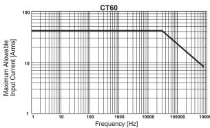
Figure 4. Derating of Primary Current by Frequency
