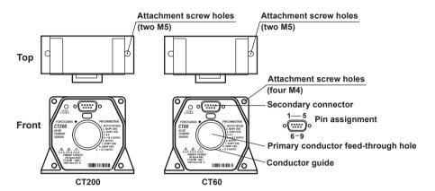
Figure 1. Names of Parts and Pin Assignments
