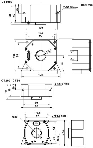
Unless otherwise specified, tolerances are ±3% (however, tolerances are ±0.3 mm when below 10 mm). Figure 5. External Dimensions
