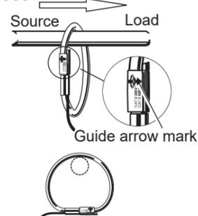
Reference test position of the conductor for 96065
