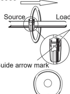
Reference test position of the conductor for 96066
