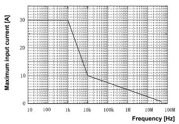
Figure 2 Derating according to frequency
