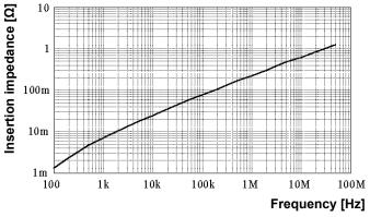
Figure 3 Input impedance (typical)
