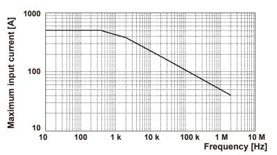
Figure 2 Derating According to Frequency
