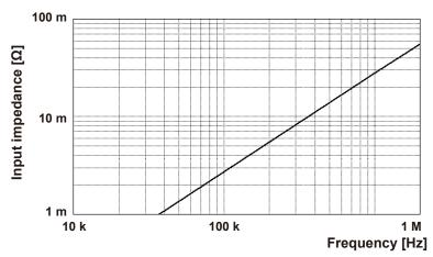
Figure 3 Input Impedance (Typical Characteristics)
