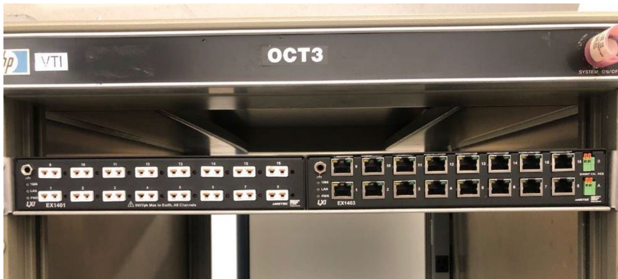
Figure 2-4: EX1403A/EX1403 Sample Rack MOUNT KIT Installation
