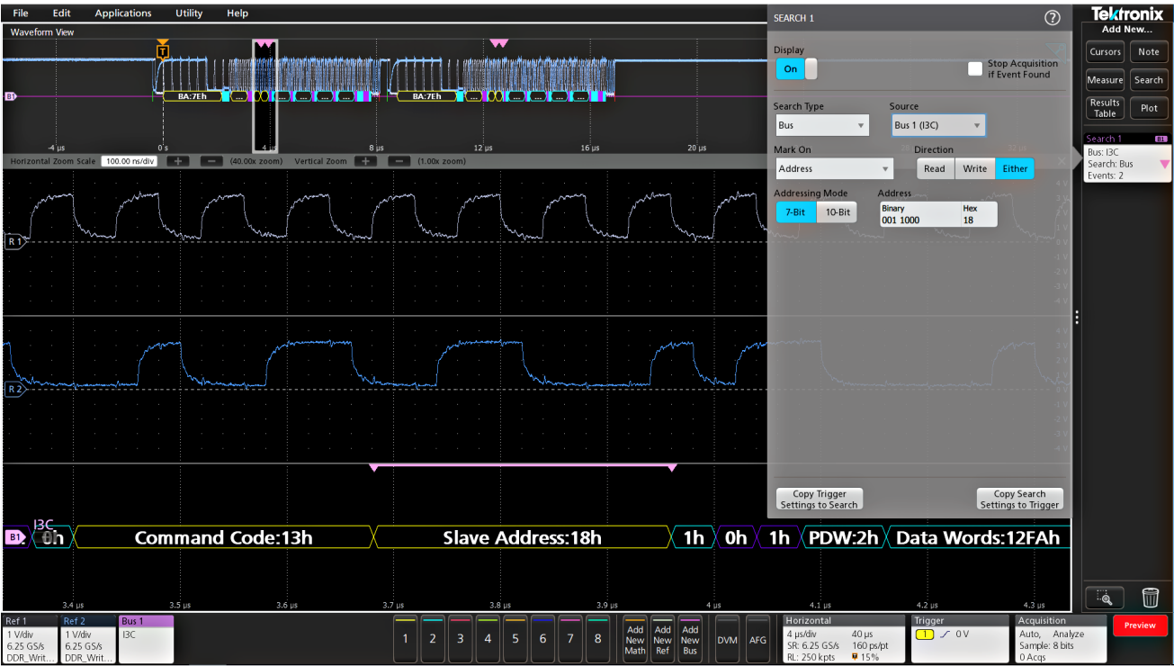
Searching on a specific data pattern on the I3C bus and automatically searching on Sync.
