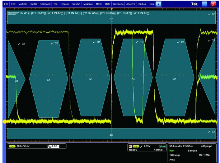
Boolean logic trigger qualification. Boolean logic using logical OR allows the user to simultaneously monitor each bit and capture the occurrence of an anomaly at any point in the acquisition.
