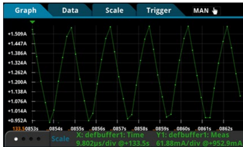
Figure 42: Inductor current linearity results at 4 ohms
