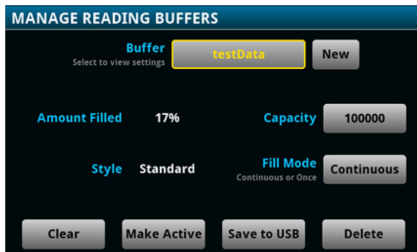
Figure 117: MANAGE READING BUFFERS window
