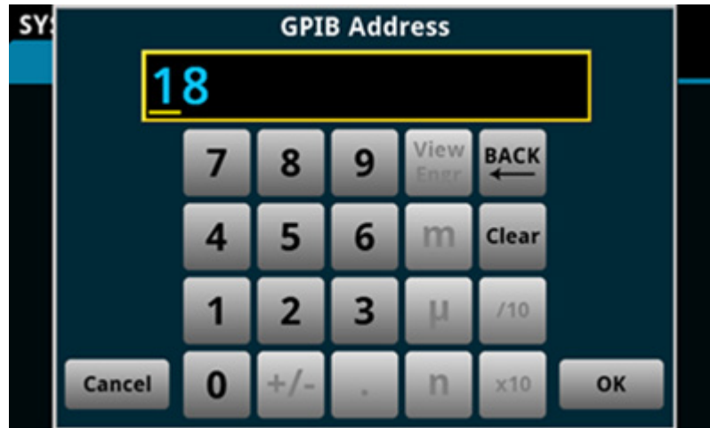
Figure 3: Front-panel keyboard for GPIB Address entry
