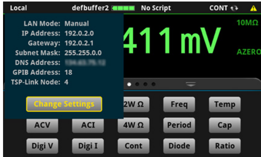
Figure 7: Communications indicator expanded
