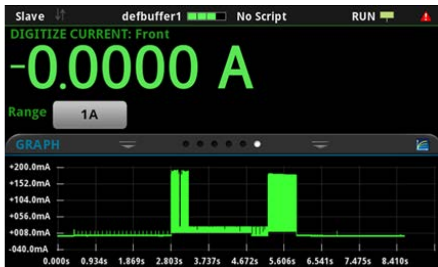
Figure 47: Subordinate node current waveform
