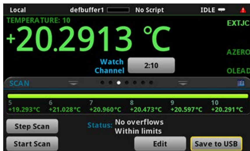
Figure 40: DMM6500 final temperature measurement
