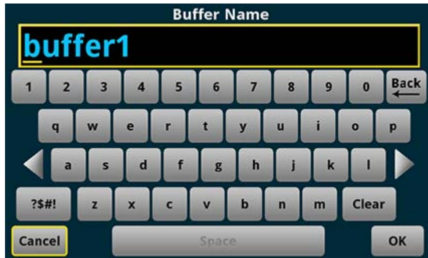
Figure 3: DMM6500 front-panel keyboard for information entry
