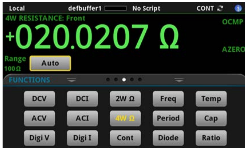
Figure 36: 4-wire resistance test results
