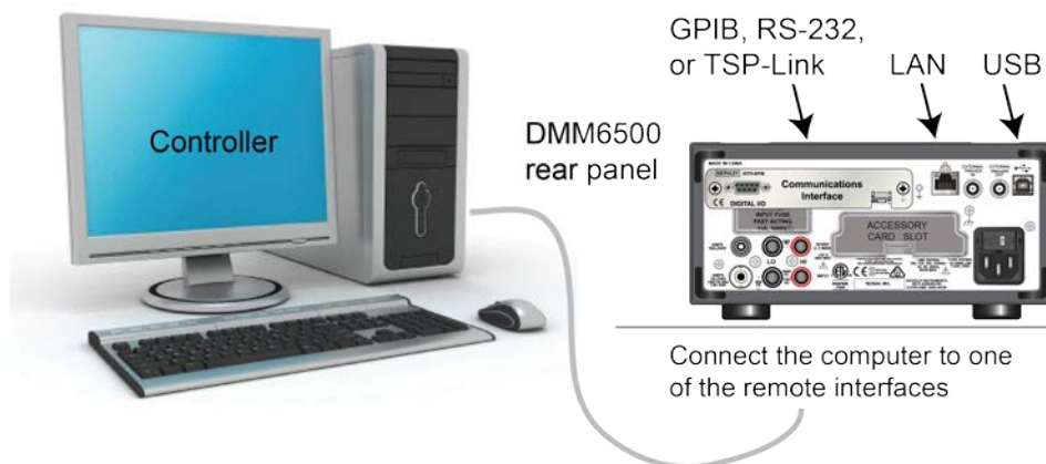
Figure 15: DMM6500 remote interface connections
