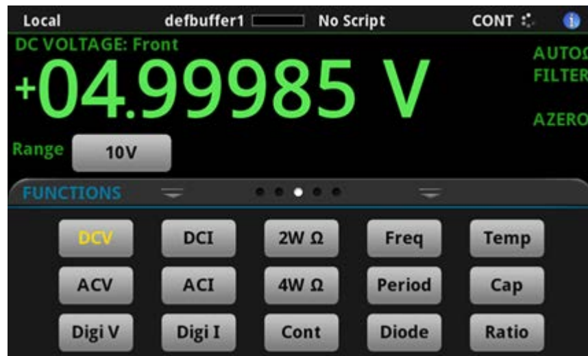
Figure 33: DC voltage high accuracy test results
