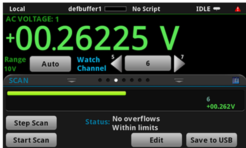
Figure 120: SCAN Swipe screen - edit scan settings
