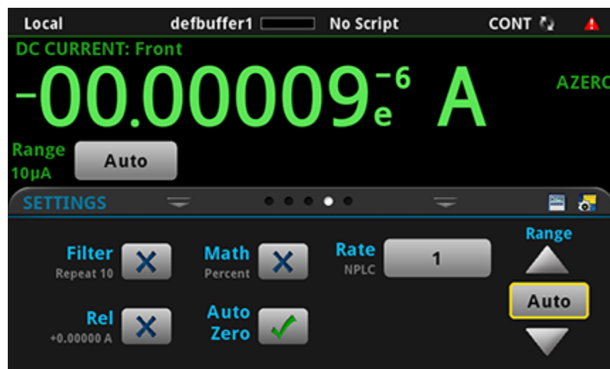
Figure 56: DMM6500 exponent display format
