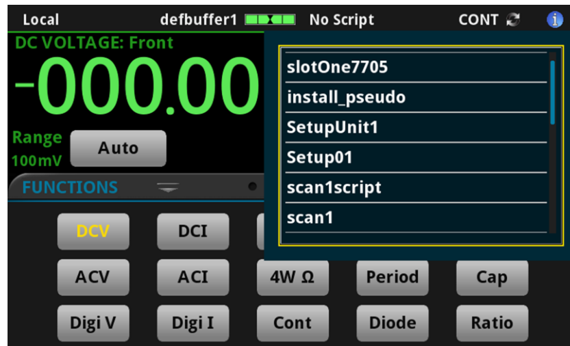
Figure 34: DMM6500 active script indicator
