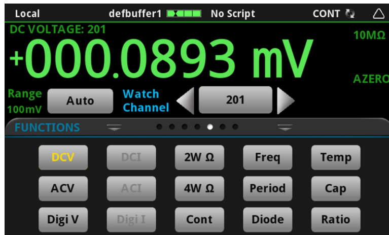
Figure 29: DMM6500 home screen - rear
