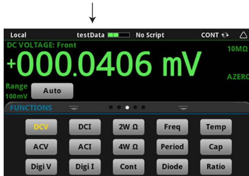
Figure 127: Active buffer indicator
