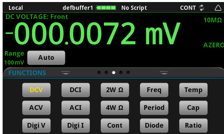
Figure 28: DMM6500 home screen - front
