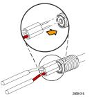
Connect the Y-lead to MMCX adapter 1
