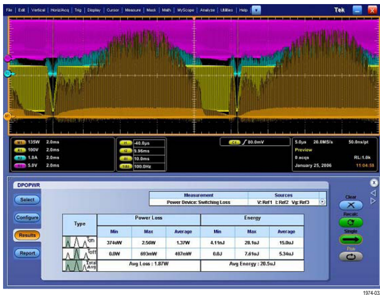
Figure 5: Switching loss results display
