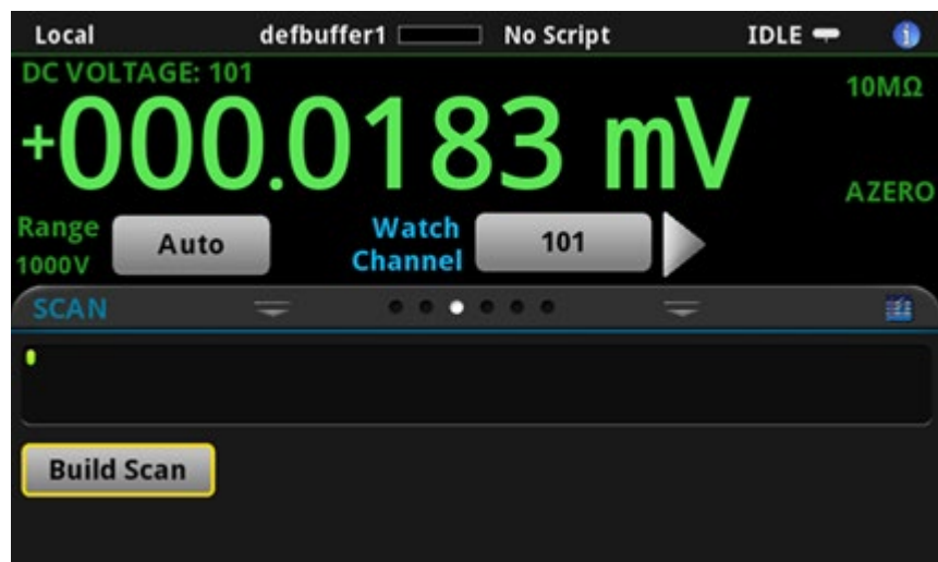
Figure 46: SCAN swipe screen - initial view
