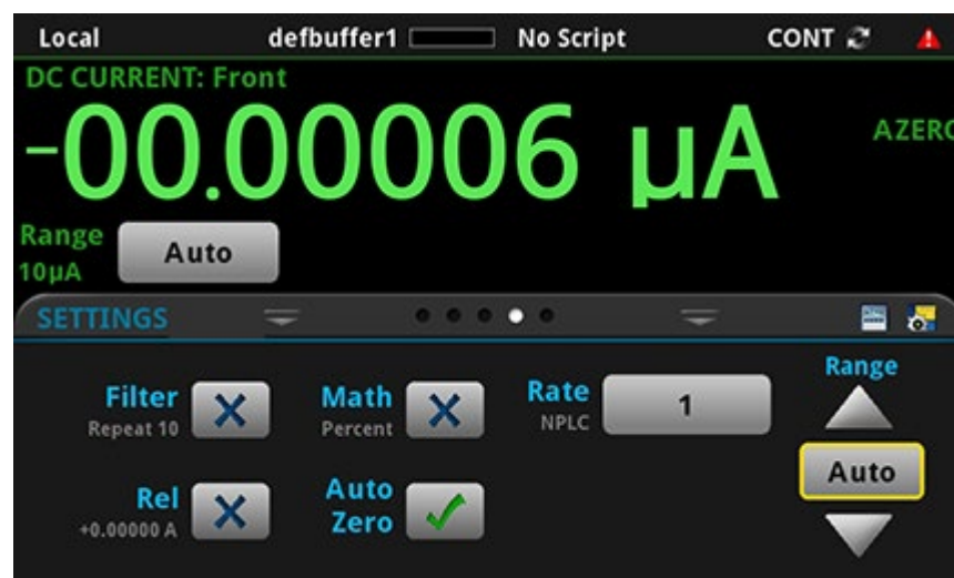
Figure 57: DAQ6510 prefix display format
