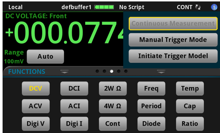
Figure 35: Trigger mode indicator
