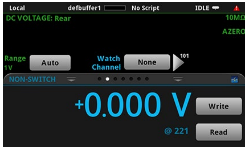
Figure 45: DAQ6510 NON-SWITCH swipe screen
