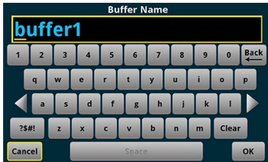
Figure 26: DAQ6510 front-panel keyboard for information entry
