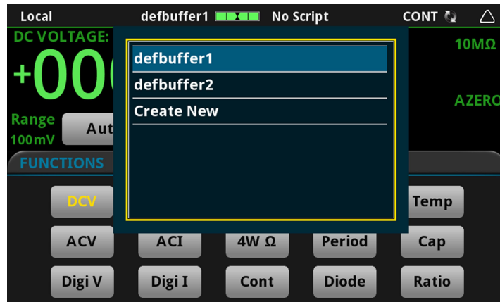
Figure 33: Active buffer indicator menu - front
