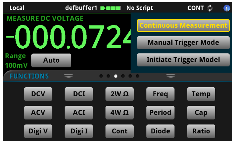
Figure 60: Trigger mode indicator
