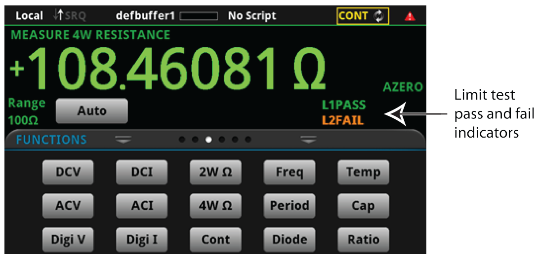
Figure 86: Limit test pass and fail indicators
