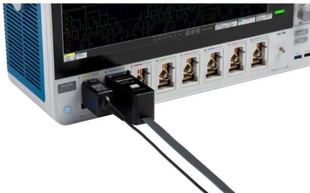
Figure 1: FlexChannel technology enables the ultimate in flexibility. Each input can be configured as a single analog or eight digital channels based on the type of probe you attach.
