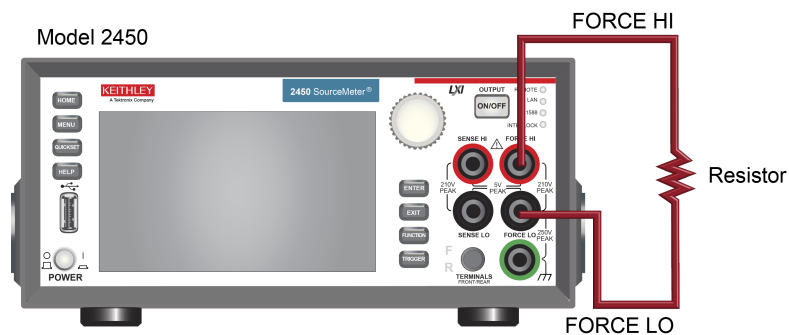
Figure 19: Model 2450 2-wire front-panel connections
