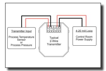
Typical loop with 2-Wire Transmitter
