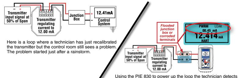
a leakage of 0.45 mA - approximately the offset seen in the control room. He walks the loop and opens a junction box releasing a stream of water. The loop is again in control.
