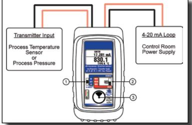
Typical loop with PIE 830 in place of Transmitter
