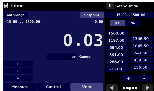
Figure 6.4.1.2.3-B – DUT Pressure Value Entry
