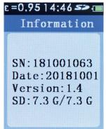
The setup option **INFO** displays the camera serial number, date of manufacture, firmware version and size of the fitted micro SD card.
