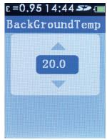
The BGT setting allows the user to set the background temperature.
