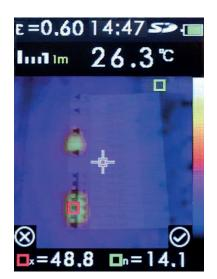
Unclip and retract the lens cover. Point the camera at the object or area of interest and pull the measurement trigger.
