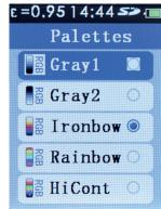
The **PLT** setting allows a user defined choice of the thermal display palette on the LCD displayed images.
