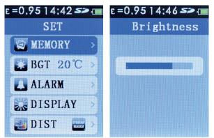
The DISPLAY setting allows the user to adjust the LCD brightness.
