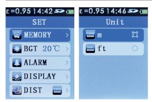
Press the **MENU** button to enter the setup menu. Use the **UP / DOWN** navigation buttons to highlight the DIST option. Press the **Enter** button.
