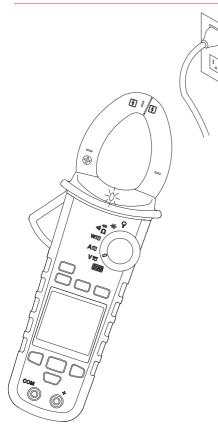
The red diamond shape LED will Illuminate if an electric field has been detected by the jaw.
