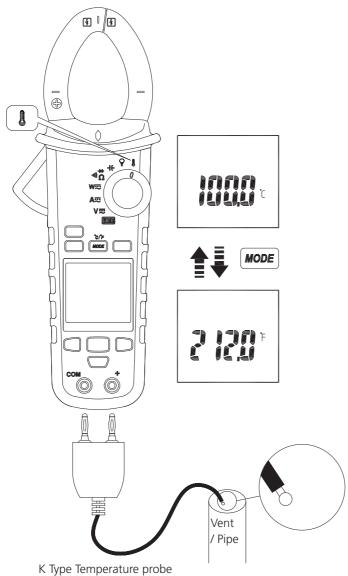
Do not take any high voltage measurement prior to making a temperature measurement as °C/°F measurement accuracy may be affected.
