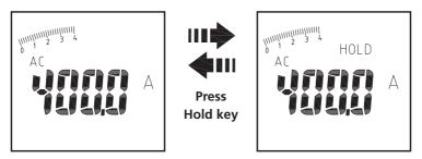
**SMART HOLD:** The meter will beep continuously and the display will flash if the measured signal is larger than the displayed reading (for V, A, W)
