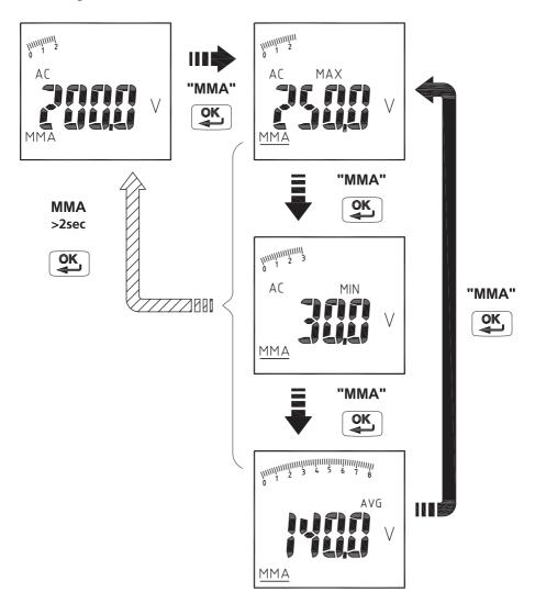
**NOTE:** Press the HOLD key in Max/Min/AVG mode to stop the meter updating the maximum, minimum and average values. HOLD mode must be turned off to continue updating values.
