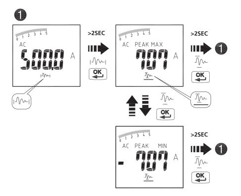
In PEAK HOLD mode, the meter will save the positive peak value and negative peak value. Positive peak value is displayed in PEAK MAX mode. Negative peak value is displayed in PEAK MIN mode.
