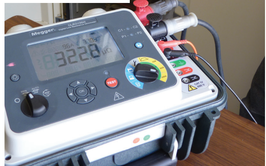
DLRO100H testing rack-mounted, 3-phase circuit breakers
