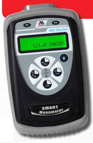
Meriam's M200LS Lab Standard Smart Manometer offers the best available pressure measurement accuracy in a portable, handheld format. The NIST traceable accuracy is typically  $\pm 0.01\%$  of F.S. and is independent of temperature effect over an operating temperature range of 59° to 86° F. Pressure ranges from 28" H<sub>2</sub>O F.S. to 500 PSIG F.S. are available.
