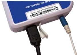
For stationary applications we strongly recommend you connect a power supply (see <u>Powering the UTRED30-WiFi</u>).
