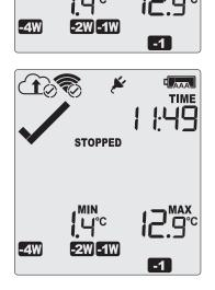
Once the logger has stopped, the last alarm status before the logger stopped will continue to be indicated with a cross or a tick symbol on the display, but the audible alarm and the alarm LED will turn off (see exception <u>below</u>).
