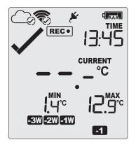
If the sensor was disconnected for a complete day, the minimum and maximum statistics for that day will show — — — on the display and — — in the list.
