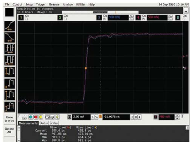
Time domain step response of N2796A (with Keysight MSO9404A)
