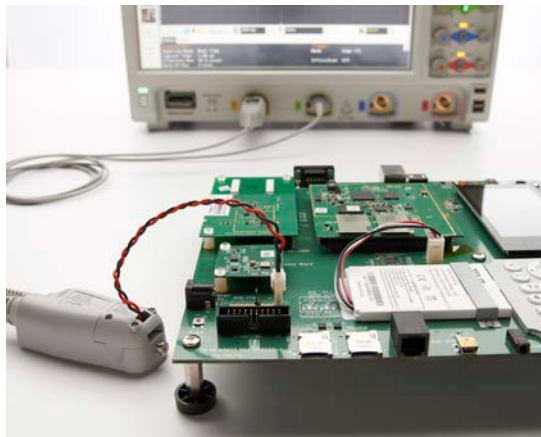
N2820A high-sensitivity 2-channel current probe
