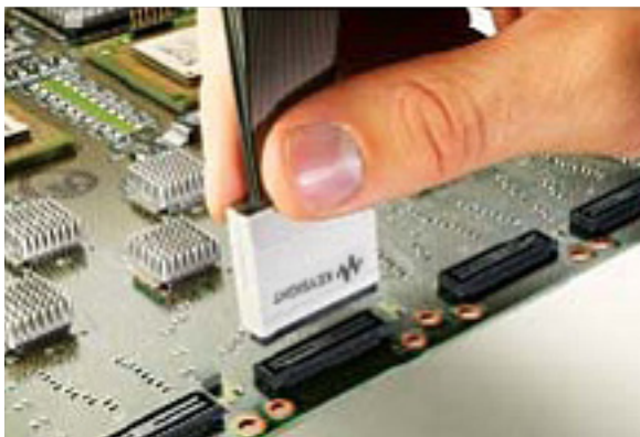
E5385A 34-channel Samtec connector probe
