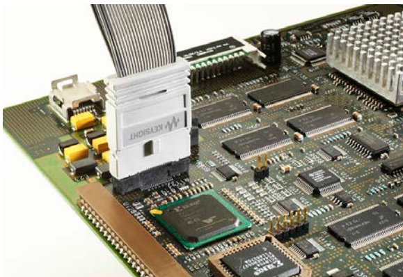
E5346A 34-channel Mictor connector probe
