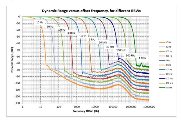
$<sup>^{\</sup>rm 1}$  For 1 MHz RBW, the sideband observed may degrade the dynamic range to -70 dBc
