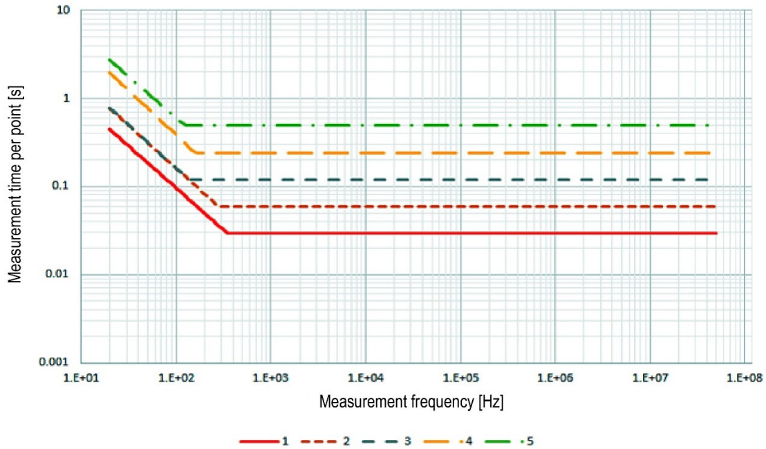
Figure 4. Measurement time (Option 050/ 030/ 020/ 010 without option 001, Typical)
