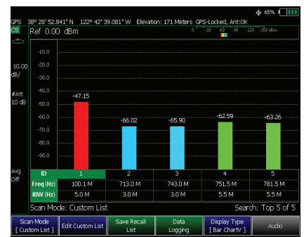
Scan up to 20 channel simultaneously with channel scanner option
