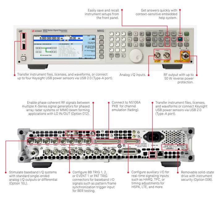
Note: The MXG and EXG X-Series vector signal generators have the same connector layout.
