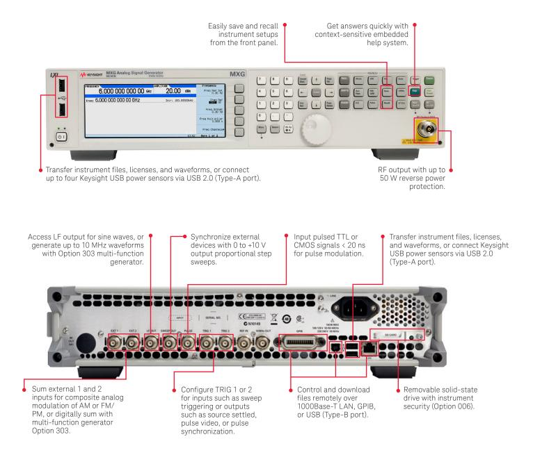
Note: The MXG and EXG X-Series analog signal generators have the same connector layout.
