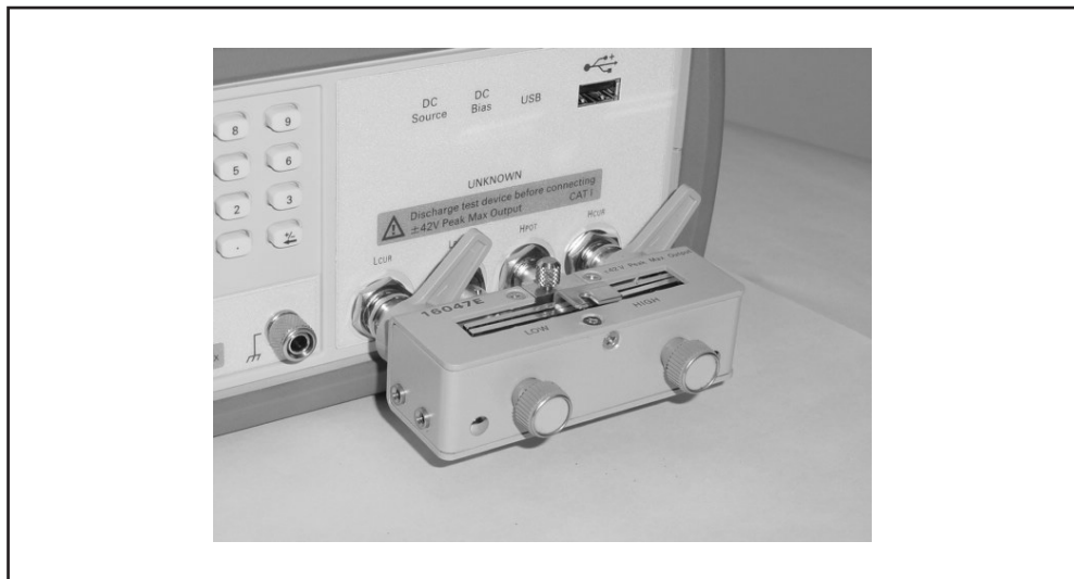
Figure 7-19 Connecting a shorting bar
