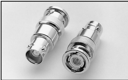
Model 6172: 2-slot male to 3-lug female triax adapter. For use in adapting Models 7065 and 2500INT inputs to 3-slot triax plugs.
