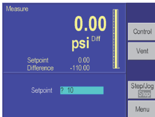
Figure 4-5. Entering Pressure in the Main Menu
