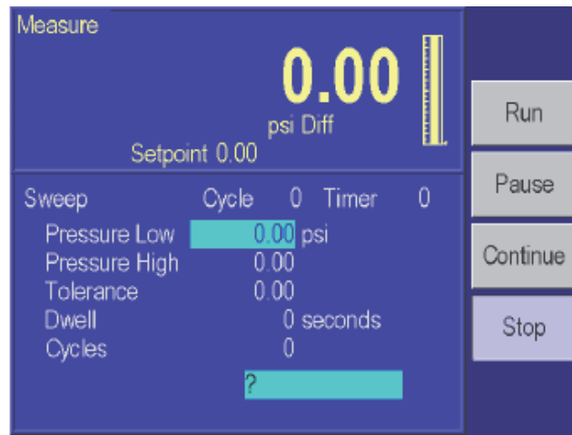
Figure 4-25. Menu | Test | Sweep - Menu
