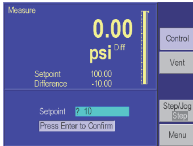
Figure 4-6. Control Mode in Main Menu
