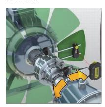
Rotate shaft and take 3rd measurement when green
