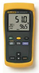
Fluke 51 Single Input Digital Thermometer
