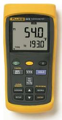
Fluke 54 Dual Input Digital Thermometer with data logging
