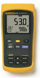
Fluke 53 Single Input Digital Thermometer with data logging
