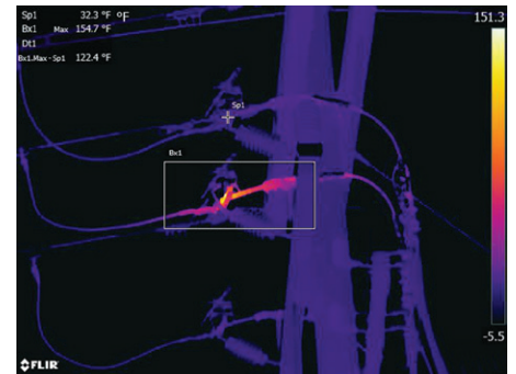
The center phase of this gang-operated switch at PUD 3’s Pioneer substation was failing. If not repaired the switch would have burned up, cutting power to about 1,600 customers and posing a safety hazard to linemen who had to operate it.
