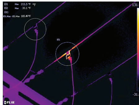
The center-phase hot tap is showing imminent failure. This hot line-clamp, or bail, connects two circuits together. A poor connection on the line clamp is causing heating on the primary line. Had it failed, 2,250 customers would have lost service.
