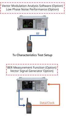
**Rx Sensitivity Test Setup**
