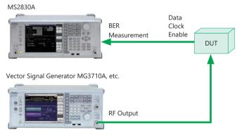
BER Measurement Setup Example (using external vector signal generator) The versatility of the MS2830A series is tailored easily to the application by installing modules in expansion slots.
