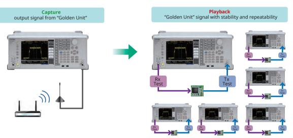
Use "Golden Unit" Signal for Manufacturing Test and Calibration
