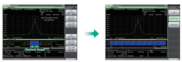
Playback any Desired Section of Captured Waveform
