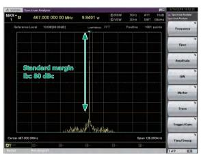
Spurious Emissions (out-of-band) Measurement Example
