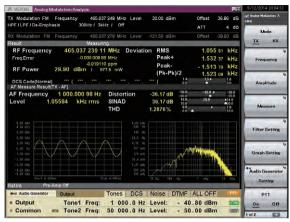
Example of AF Signal Output (bottom) and FM Signal (top) Measurement
