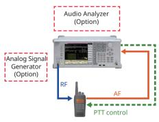
**Rx Sensitivity Test Setup**
