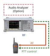
**Tx Characteristics Test Setup**
