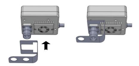
Figure -1. Installation of the MN8861A Stabilizing Bracket
