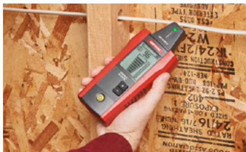
Trace energized and de-energized wires
