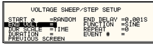
Figure 5-12: VOLTAGE SWEEP/STEP SETUP Screen
