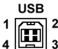
Figure 3-4: USB Connector pin orientation.
