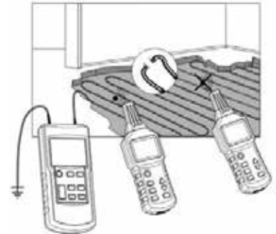
Detects breakers in radiant heating systems
