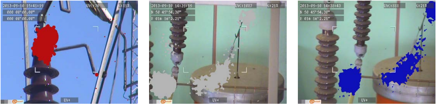
Examples of UV discharges. User can opt to show in red, white, or blue rendering against target image
