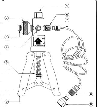
The system is a portable dual source of vacuum and pressure. Each system incorporates a vacuum / pressure selector, a volume control for fine adjustment and adjustable stroke to provide over pressure protection.
