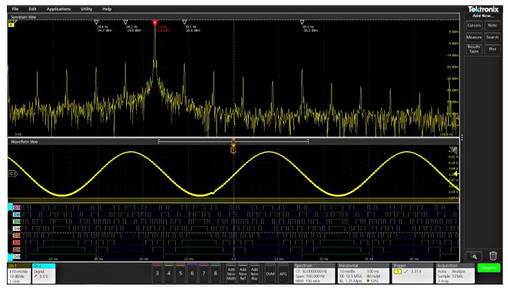
Beyond just analog and digital, FlexChannel inputs include Spectrum View. This Tektronix-patented technology enables you to simultaneously view both analog and spectral views of your signal with independent controls in each domain. For the first time ever, oscilloscope-based frequency-domain analysis is as easy as using a spectrum analyzer while retaining the ability to correlate frequency-domain activity with other time-domain phenomena.
