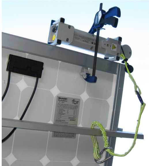
Figure 20. SolSensor tool lanyard secured to a racking member.
