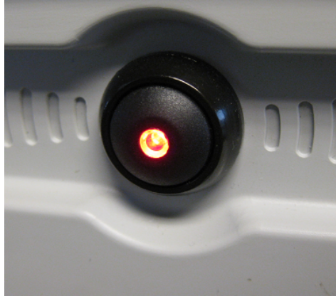
Figure 25. SolSensor pushbutton with LED lit. LED blinks until wireless network is established, after which it remains on.
