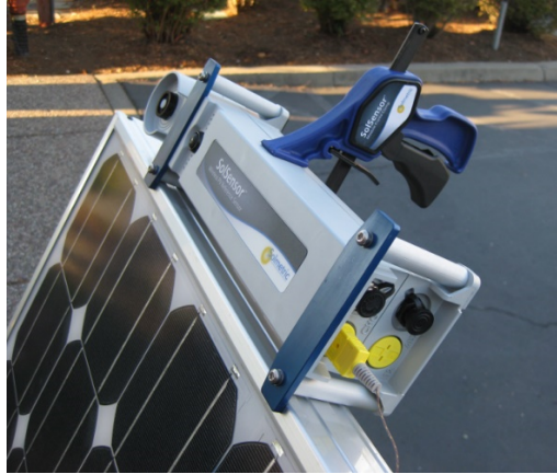
Figure 19. SolSensor mounted on the frame of a PV module
