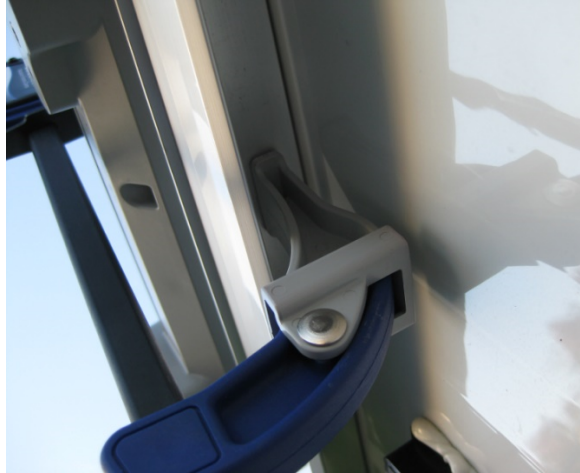
Figure 22. Tip of frame clamp properly seated on inside surface of module frame
