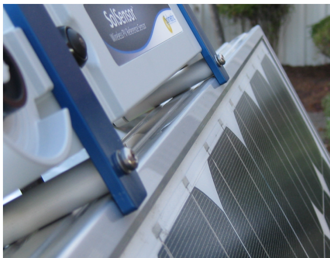
Figure 21. SolSensor correctly seated along the upper horizontal leg of the module frame.
