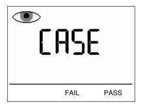
Recording a fail result will cause the tester to skip testing and go straight to the end of test options.
