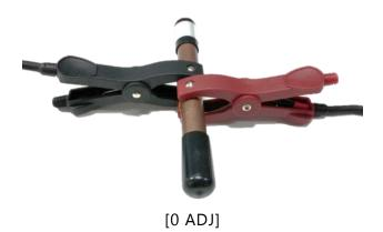
• As shown above, use the adjust kit. Clamp each jaw of test probes onto the adjust kit to conduct the 0 ADJ.
