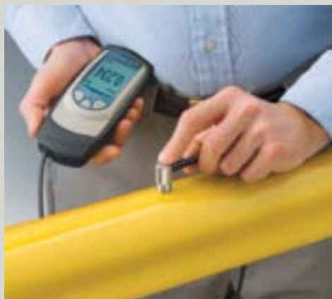
Flip Display enables right-side-up viewing whether the gage is in your hand, on your belt or on a work table
