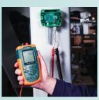
Precision "source" for calibrating process devices.
