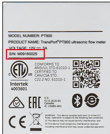
Figure 63: Transmitter Serial Number
