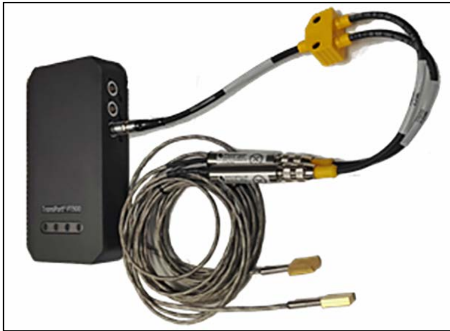
Figure 47: Energy Cable Connection (Right Side)
