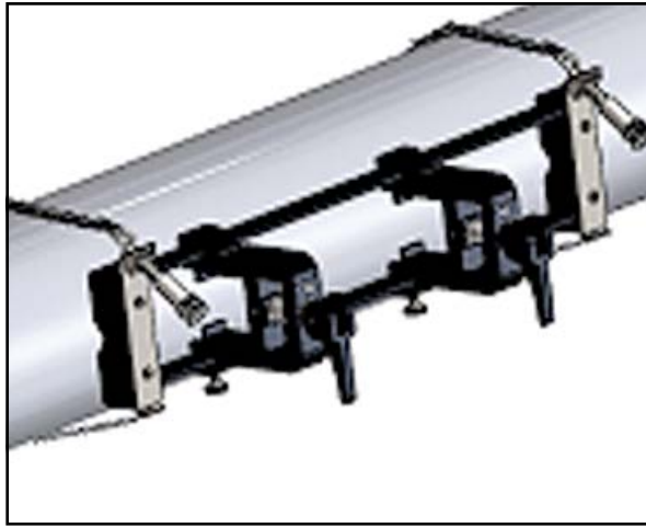
Figure 15: Fixture With Chains Installed
